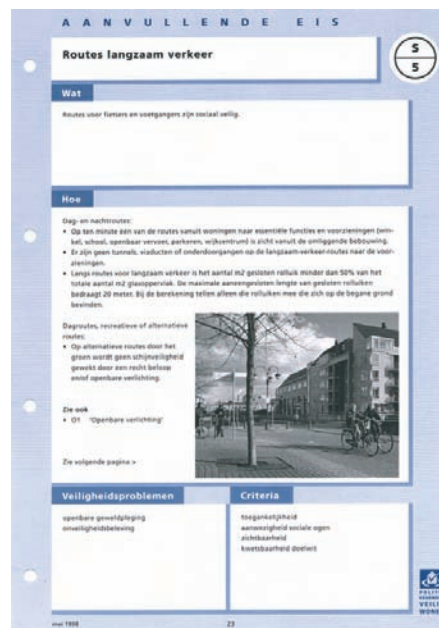
Figure 2: An example of one of the requirement sheets, at the top: 'what' (performance) and 'how' (specification) 23
